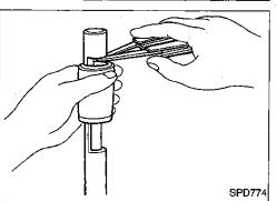
Select the correct thickness of pinion bearing preload adjust-9. ing washer using a standard gauge of 3.5 mm (0.138 in) and your J34309-101 feeler gauge. The exact measure you get with your gauges is the thickness of the adjusting washer required. Select the correct washer.
