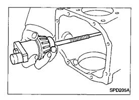
17. Remove the J34309 pinion preload shim selector tool from the final drive housing and disassemble to retrieve the pinion bearings.
